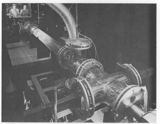
PLASMA ACCELERATOR produces tremendous velocities in small masses of materials and enables study of the interaction of individual atoms with gases, with surface, and with magnetic fields. In the control room are D. M. Zagar, left, and R. L. Schellenbaum of Radiation Physics Division.
